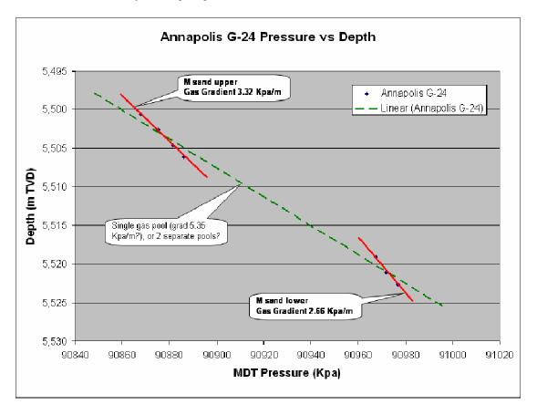
Figure 94. Annapolis G-24: Pressure versus depth plot for the M sands (MDT pressures).
