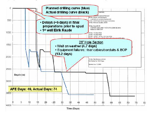
Figure 119. Drilling curve for Torbrook C-15 (AFE and actual).
