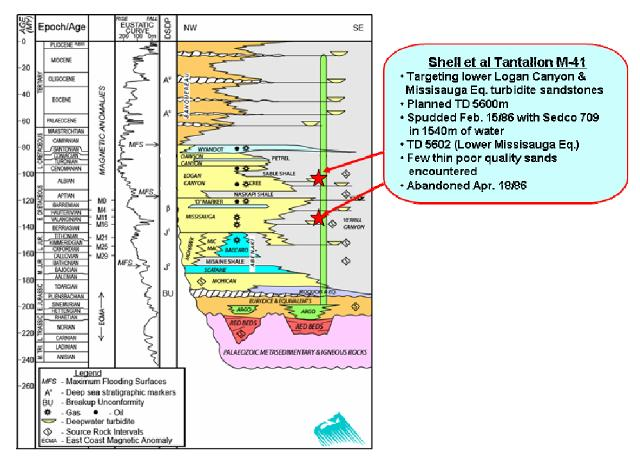
Figure 76. Stratigraphic chart showing target intervals for Tantallon M-41.
