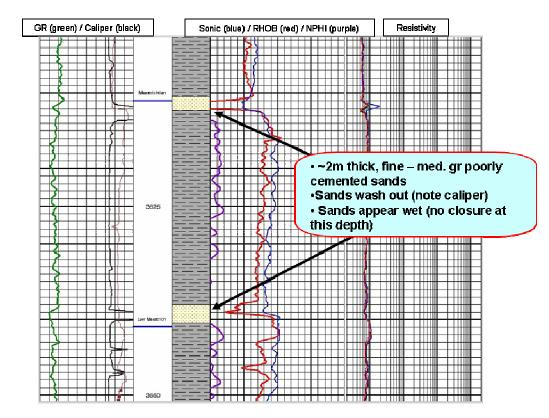
Figure 124. Balvenie B-79: Well logs from Late Maastrichtian sands.
