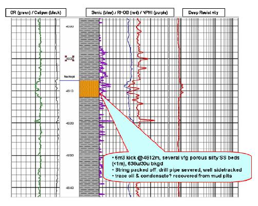
Figure 136. Weymouth A-45: Well logs from Naskapi-equivalent (Aptian?) "kick zone".
