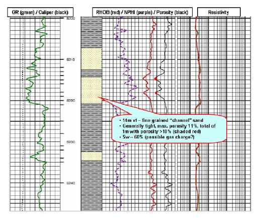
Figure 79. Tantallon M-41: Well logs from Late Hauterivian sands (Missisauga equivalent).
