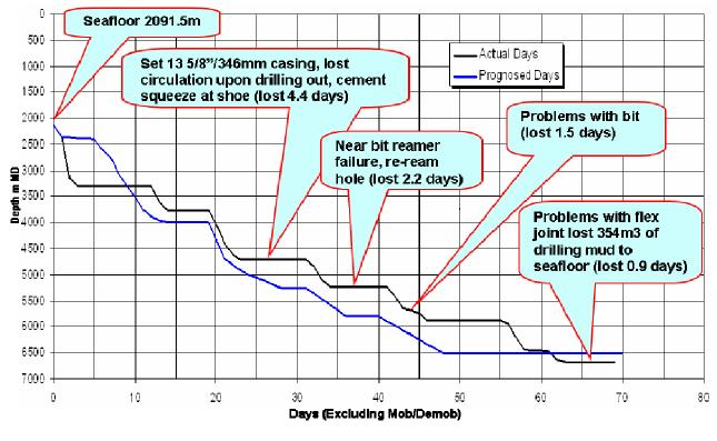
Figure 155. Drilling curve for Crimson F-81 (AFE and actual).
