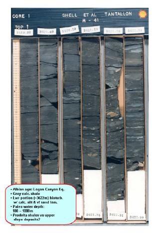
**Figure 80.** Tantallon M-41: Portion of Core #1 (3600.0 – 3627.0 m, 23.5 m recovered).
