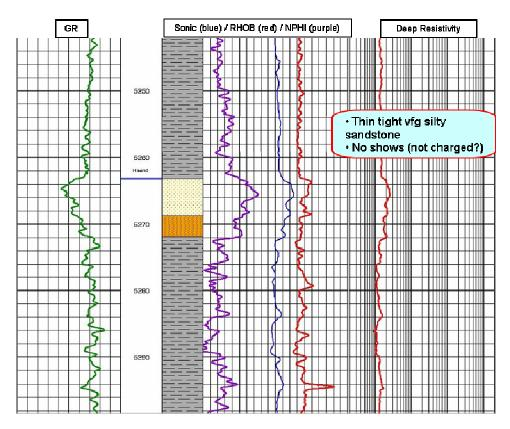
Figure 148. Crimson F-81: Well logs from the "H" sand interval (Early Barremian).
