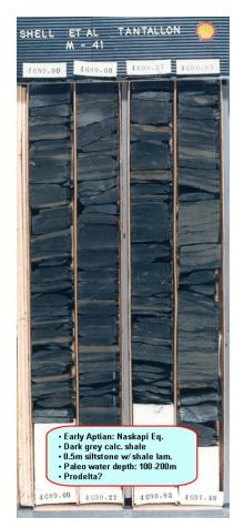
**Figure 81.** Tantallon M-41: Portion of Core #2 (4689.0 – 4717.0 m, 28.0 m recovered).
