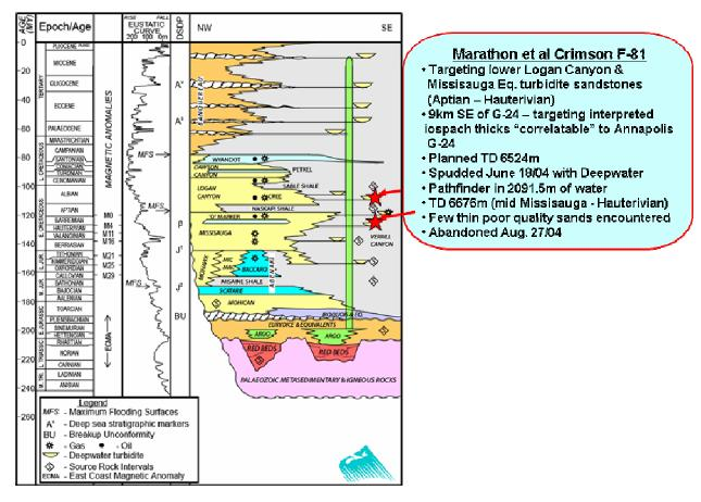
Figure 142. Stratigraphic chart showing target intervals for Crimson F-81.
