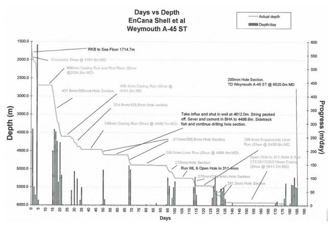
Figure 141. Drilling curve for Weymouth A-45 (actual).
