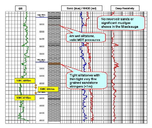
Figure 137. Weymouth A-45: Well logs from target Missisauga interval (Barremian – Valanginian?).
